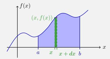
$$\int_{a}^{b} f(x) dx = \text{area under curve}$$
