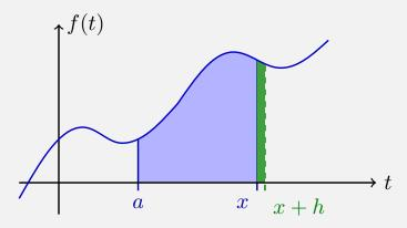
$$\frac{d}{dx}F(x) = \frac{d}{dx} \int_{a}^{x} f(t) dt = \lim_{h \to 0} \frac{\int_{a}^{x+h} f(t) dt - \int_{a}^{x} f(t) dt}{h}$$
